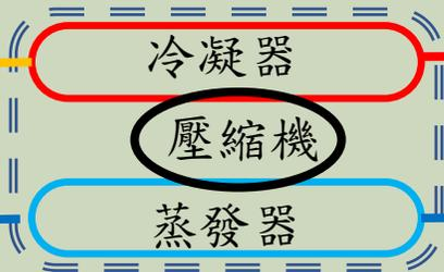
$$\text{冷媒熱負載 } q_r = \text{冰水熱負載 } q_{chw} + \text{壓縮機之壓縮功 } P_{comp}$$
